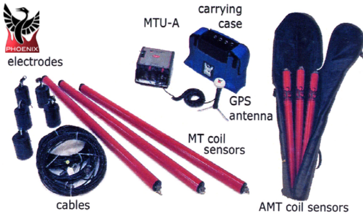
Figure 1. Phoenix MTU-A equipment.
