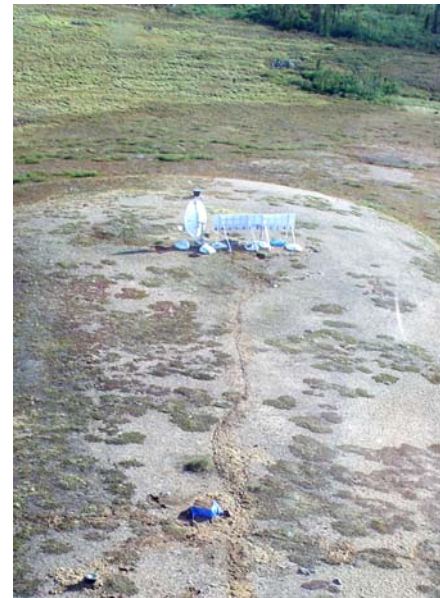
Figure 3. Observatory MT deployment at seismograph station.
